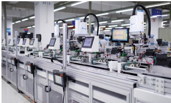
SCARA Robot with machine vision system for a function test of AC motor drives in China
